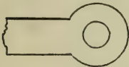
Fig. 170.—One end of an eye-bar used in tension members of bridges and roofs.
